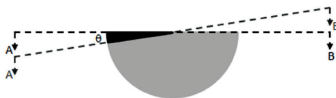
Fig. 2: The Tilting of Balance Beam by Angle ( \theta )
