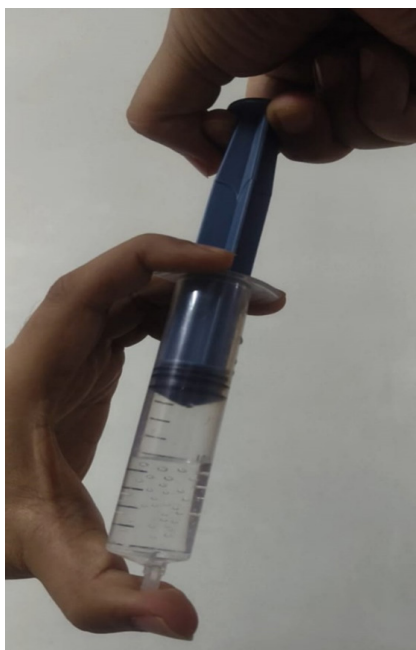
Figure 6: Demonstration of boiling of water below 100 degrees Celsius by reducing pressure
