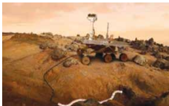
The researchers envisage using the rover to navigate over large distances, after which the snake robot can detach itself and crawl into tight, inaccessible areas. (Credit: Image courtesy of SINTEF)
