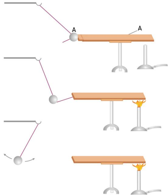
C.V. Raman's Experimental Demonstration on Death of Magnet (demagnetisation) by heating to Curie point
